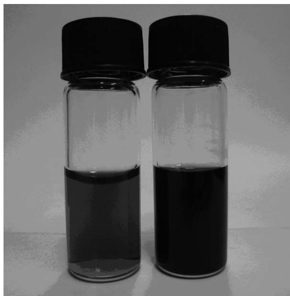
Figure 4. Photographs of GO dispersed in water (left) and DED-GO dispersed in dichloromethane (right). Concentration: 0.25 mg/mL.
